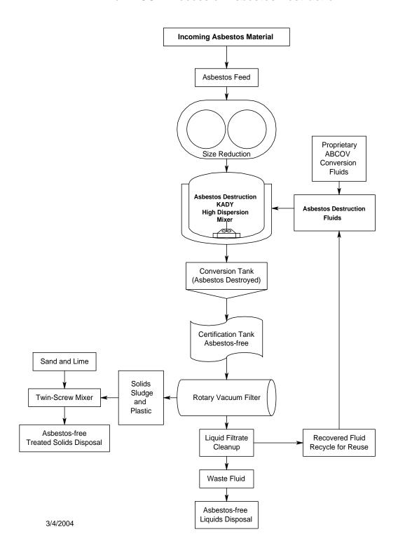
**2.2 Process Chemicals.** Materials for the process chemicals are provided in Appendix A. The ABCOV method of asbestos destruction is generally based upon the reaction of fluorides in the proprietary reagent identified as "ABCOV-C" with the silicon in the asbestos crystal to destroy the physical structure of the mineral. Other chemicals may be used to support or catalyze the reaction.
